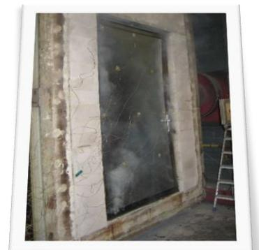
IFC has established principles, based upon extensive experience of testing steel doors for fire resistance in both directions of exposure. These principles define which orientation is 'the weakest direction' for steel doors.
